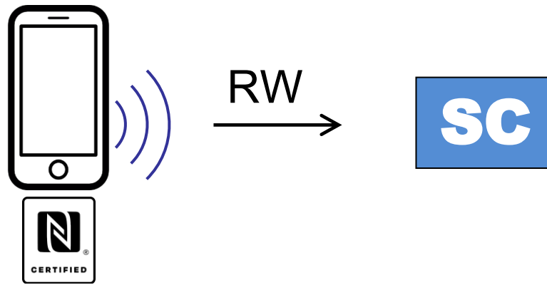
Figure 7: NFC Forum Device in NFC Forum Reader/Writer Mode Communicating with a SC
