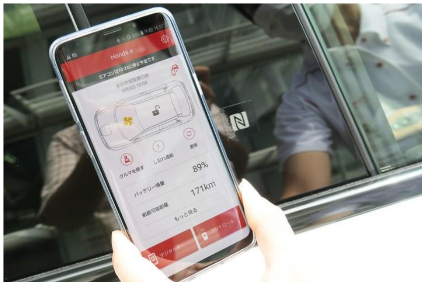
Digital Key demonstration by tapping smartphone to the NFC on the center pillar
