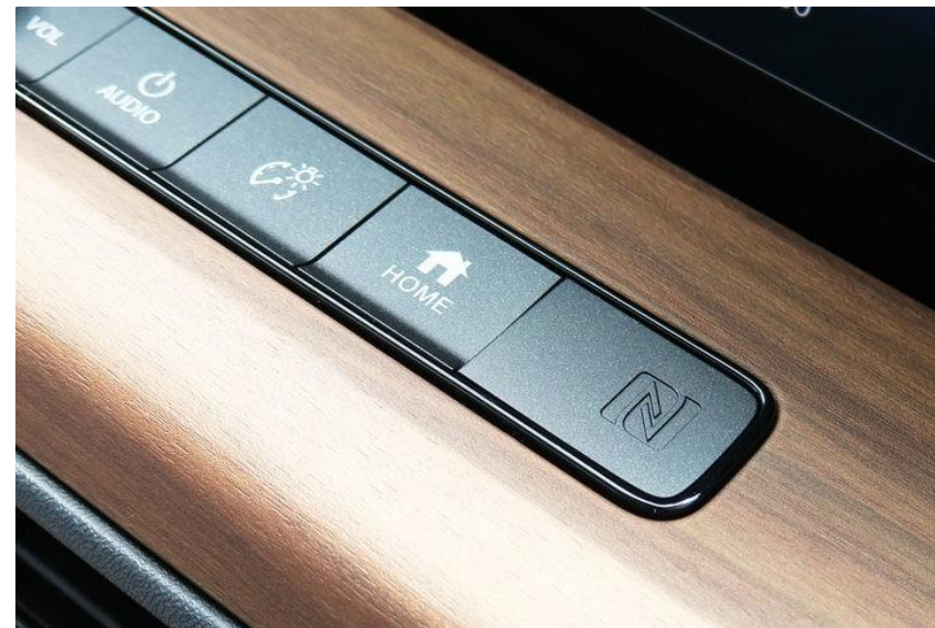
NFC sensor on the dashboard for user authentication
