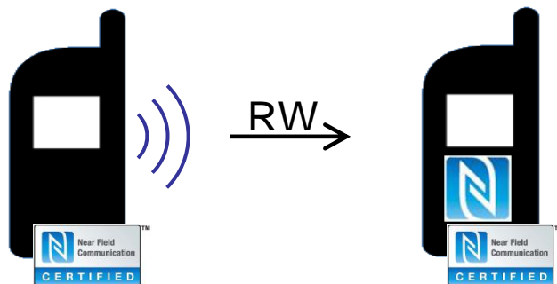
Figure 7: NFC Forum Device in NFC Forum Reader/Writer Mode Communicating with an NFC Forum Device in NFC Forum Card Emulation Mode
