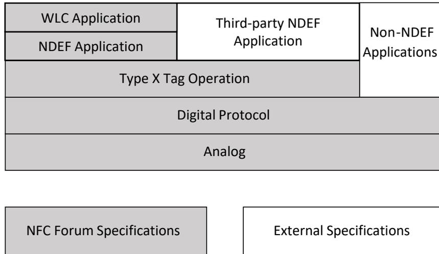
**Figure 11: Reader/Writer Mode Architecture**
