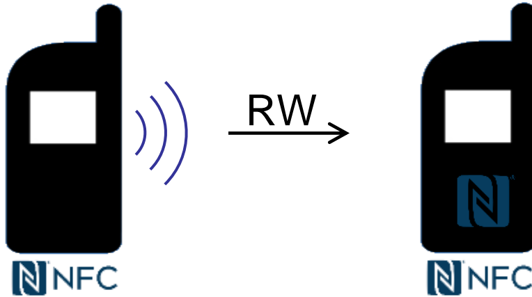
Figure 4: NFC Forum Device in NFC Forum Reader/Writer Mode Communicating with an NFC Forum Device in NFC Forum Card Emulation Mode
